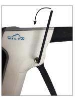
**2.** Rotate counterclockwise and remove the trigger bolt once loose.
