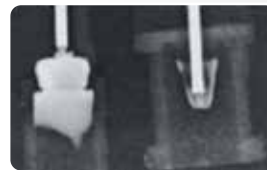
The xray shows the amount of wasted material in a conventional delivery tip (left) vs. a tip featuring MST (right)
