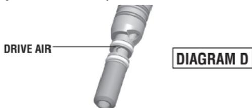
**All Impact Air 45® handpieces should be lubricated ***BEFORE*** autoclaving for maximum turbine life.**
